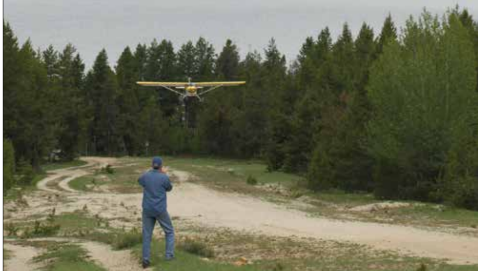
The Kitfox needs only to fly horizontal to plant itself on Deadwood Reservoir's steep airstrip.
