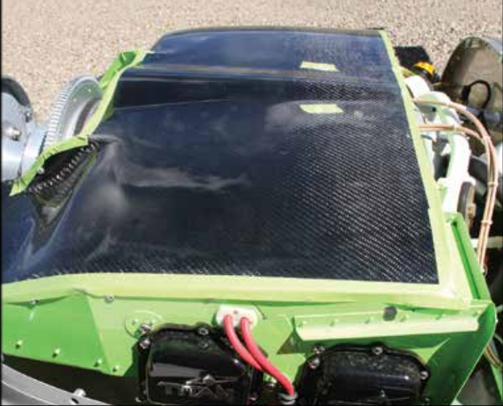
The full carbon plenum on the top of the Titan X340 makes for a clean installation. Ignore the masking tape—it's just part of the development nature of the aircraft.
