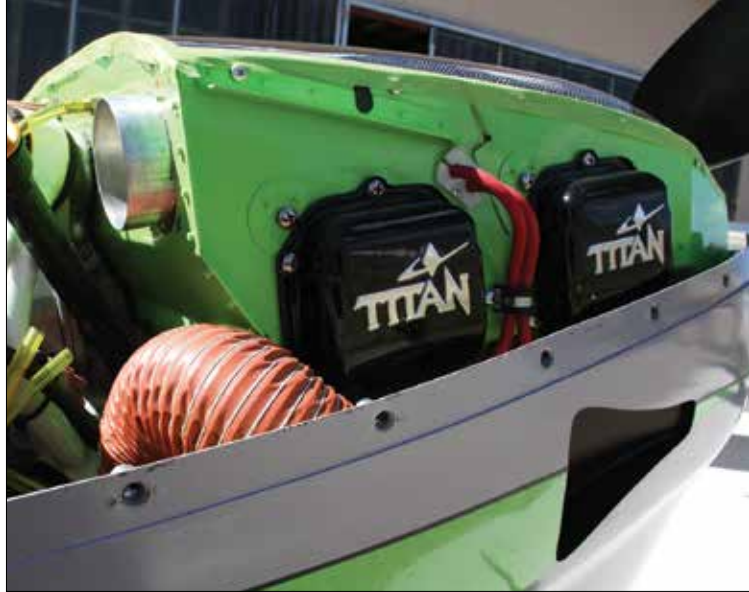
The NACA scoop on the side of the cowling feeds air to the horizontally-mounted oil cooler via a SCAT tube and duct.
