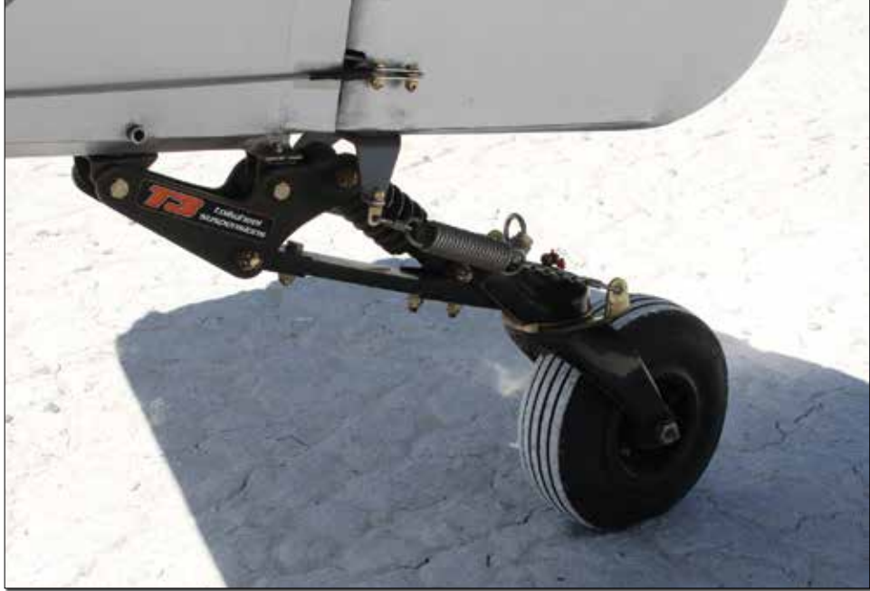
The fully articulated shock-absorbing T3 tailwheel suspension adds significantly to the nice feel when landing the STi. It absorbs the shock of a firm tailwheel touchdown without launching you back into the air.
