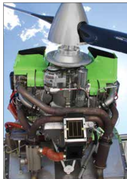
A simple airbox and filter make for a nice clean engine installation.
