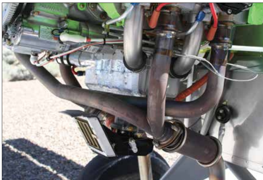
The simple exhaust system provides carb heat, but does not yet feature a cabin heat muff. It undoubtedly will in customer aircraft.
