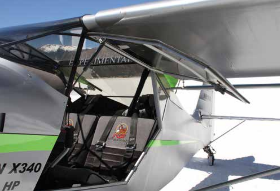
The large swing-up doors can be opened in flight, but the convex Plexiglas gives such a good view that you may not have to—the view is equally good with them closed or open.
